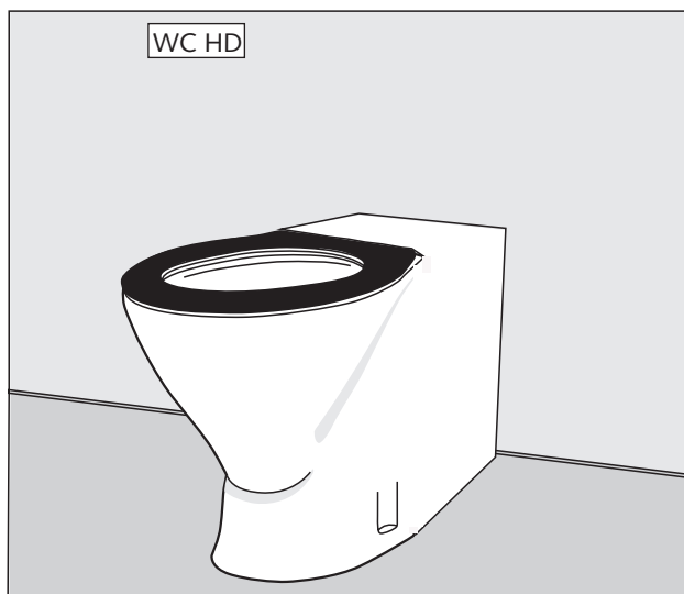
Figure 11 WC appropriate for assisted ambulant disabled/wheelchair users
